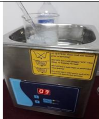
Figure.5. Ultra sonication process of MWCNT's and SiO
