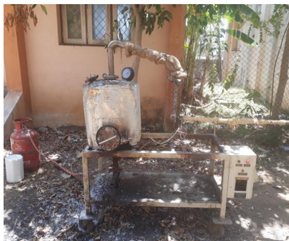
Figure 2.3: Plastic Oil Extraction Unit
