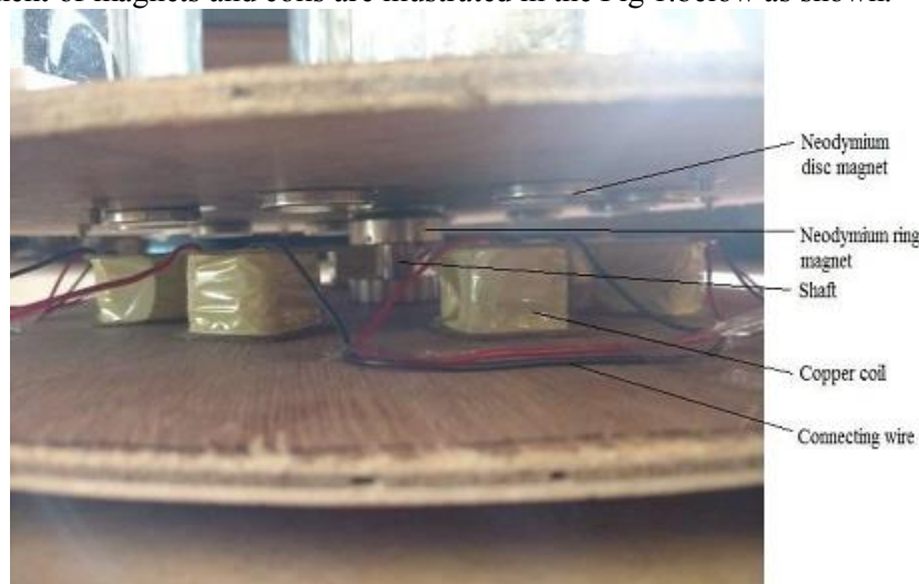
Figure 1. Levitation between Stator and Rotor
